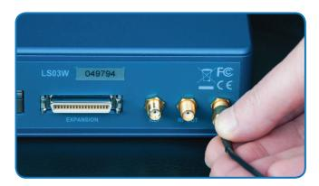
**1.** Connect the antenna to the 'RF IN' port on the rear of the LabSat 3 Wideband.
