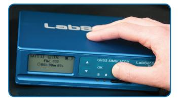
**4.** Press the 'REC' button to start recording.
