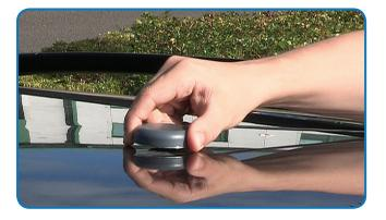
**2.** Place the antenna in the middle of the car roof.
