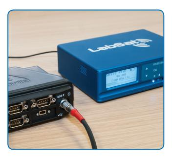
4. The Device Under Test should now be receiving the replayed satellite signal data, allowing realistic and repeatable testing to be carried out under controlled conditons.
