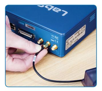
Connect the Device Under Test to the 'RF OUT' port.
