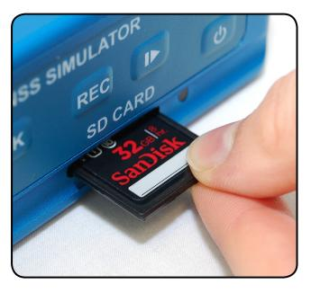
**1.** Insert SD card into the LabSat 3. Three demo scenarios are pre-loaded on the SD card.
