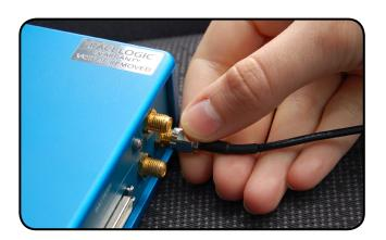
**1.** Connect the antenna to the 'RF IN' port on the rear of the LabSat 3.
