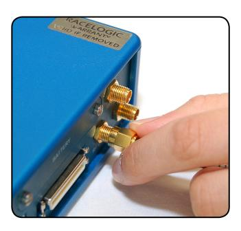
**2.** Connect the device under test to the 'RF OUT' port.
