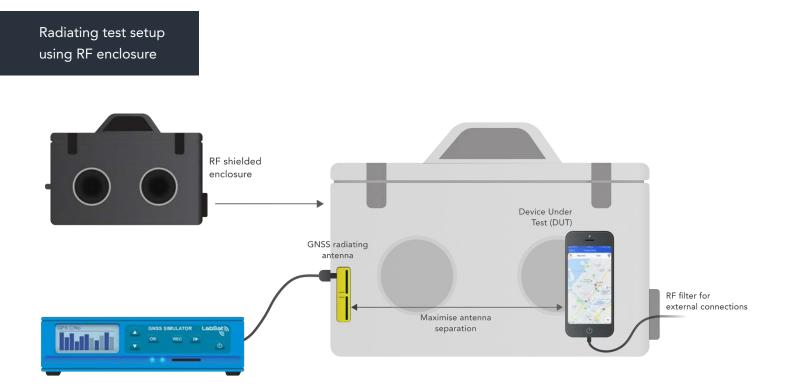
To produce a reliable and consistent test, it is critical that the device under test be consistently located, that the separation distance between the antennas is maximised (this reduces the sensitivity to placement variation) and that any connected cables be as short as possible and routed consistently between tests to minimise the risk of cable placement influencing the test results. If possible, devices should operate without any cables connected.
