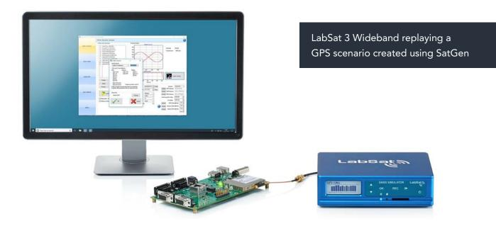
LabSat's Application Programming Interface (API) provides additional control and testing automation as scenarios can be programmed to automatically repeat or play in a set order. This improves efficiency by allowing significant testing programmes to be run continuously, without the need of human supervision.
