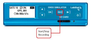
During recording, while using battery power, the GNSS monitor display will automatically revert to the record display after a short period to conserve battery power. This power save feature can be switched off but it is recommended to be left active for maximum battery life.
